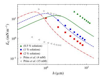
FIGURE 4. Gibbs elasticity is measured by extracting  $-d\sigma/d\ln h$  from figure 3 with (3.4). The measured values are consistent with the reported values in the literature (Prins, Arcuri & Van den Tempel 1967) but greater than the prediction of the Langmuir adsorption model in (1.2).
