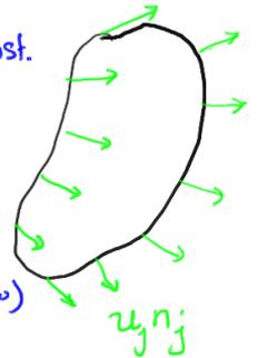
Applying divergence theorem:  $\int_{\Omega} \left[ \frac{\partial \rho}{\partial t} + \frac{\partial}{\partial x_j} (\rho u_j) \right] d\Omega = 0$
