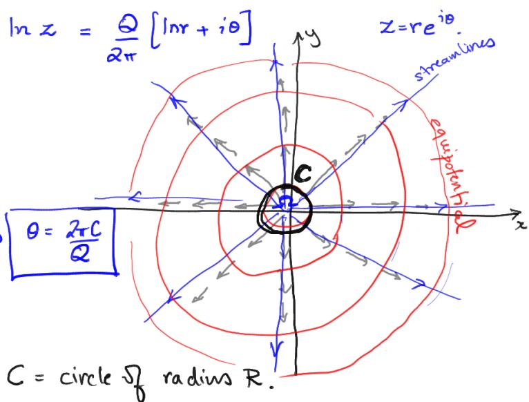
$$\text{Incompressible? } \nabla \cdot \underline{u} = \frac{1}{r} \frac{\partial}{\partial r} (r u_r) + \frac{1}{r^2} \frac{\partial u_\theta}{\partial \theta} = \frac{1}{r} \frac{\partial}{\partial r} \left( r \frac{Q}{2\pi r} \right) = 0.$$
