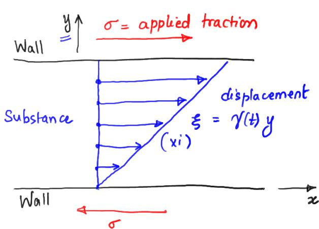
$\sigma$  = applied traction = shear stress
